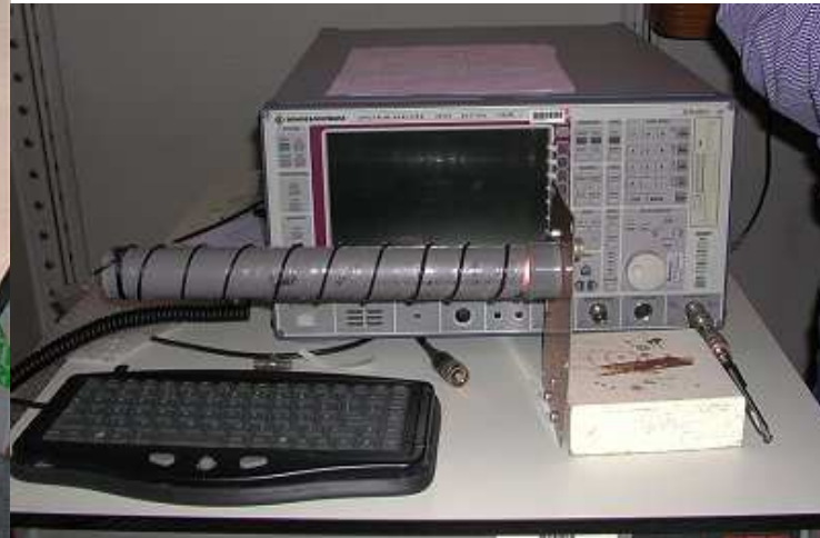
Figure 6b 'helix-in-one-hour' and Rohde & Schwarz analyser
